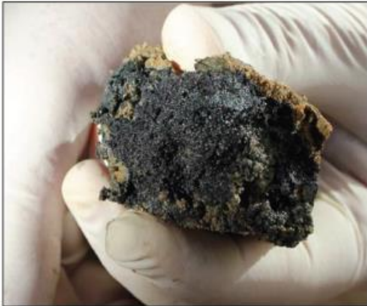
Figure 23. PlumeStop Dispersed Through Permeable Stratum
